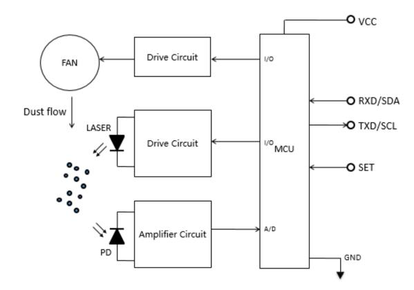
According to above Block Diagram, the air sampling of sensor is consisting of fan and drive electric, the light source is consisting of laser diode and drive electric, the detecting part is consisting of light sensitive tube and amplifying circuit.
